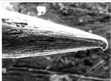
Ground needle point smoothed using the CARBOCHEM Process (enlarged approx. 190 times)
