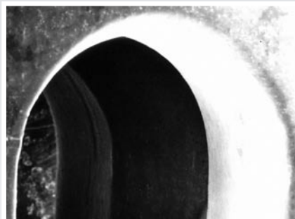
Drilled edge of two cross ports before and after deburring with the POLIGRAT Process (enlarged approx. 30 times)
