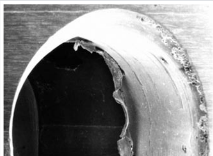
Drilled edge of two cross ports before and after deburring with the POLIGRAT Process (enlarged approx. 30 times)
