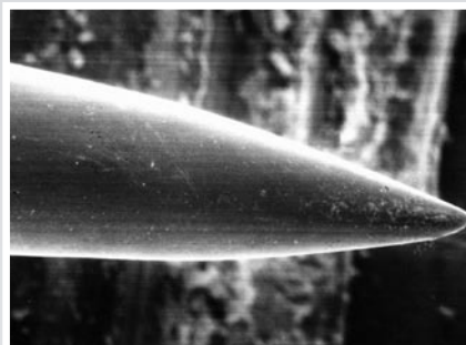
Ground needle point smoothed using the CARBOCHEM Process (enlarged approx. 190 times)
